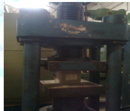
Fig1: Compressive strength testing
